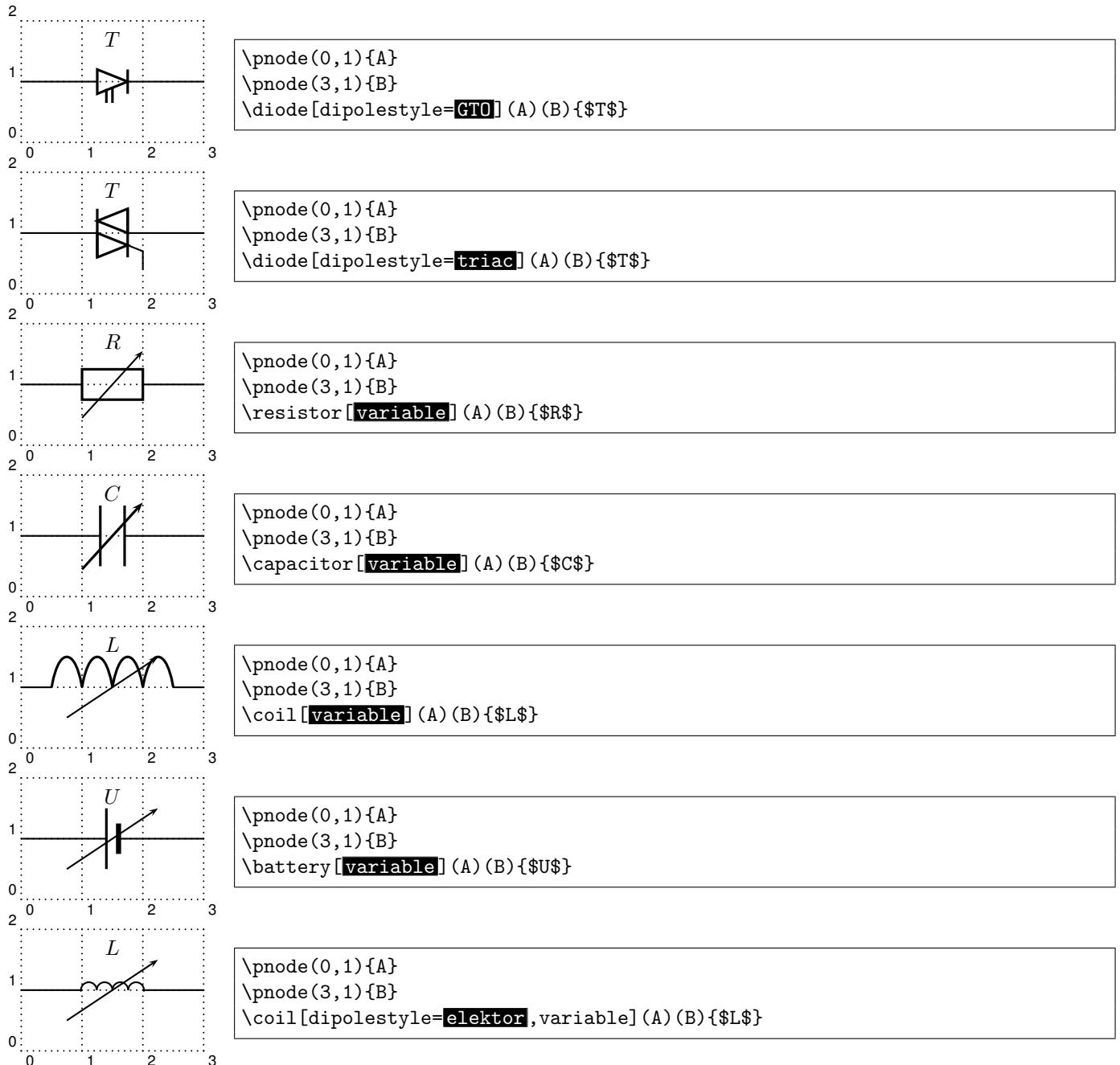
In the following example the parameter `dipolestyle` is used for a tripole and quadrupole, because the coils are drawn as rectangles and the resistor as a zigzag.
